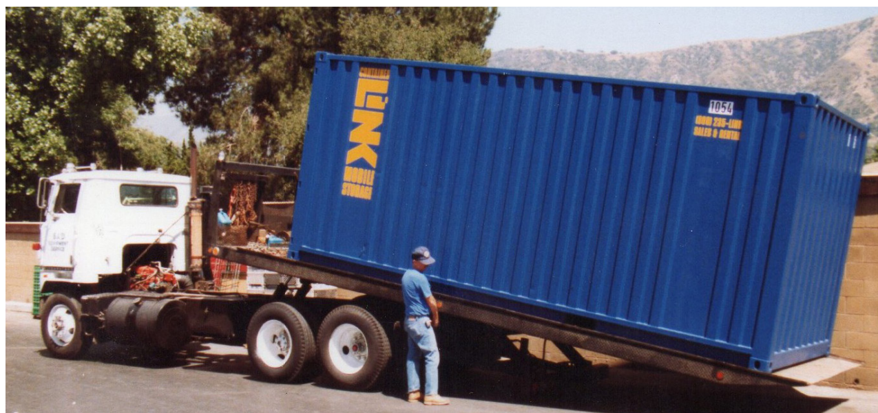
A 20ft container being delivered off-site, using a "tilting" flatbed truck. There was no need for a HIAB crane, as US clients had plenty of room in which to load/offload.
